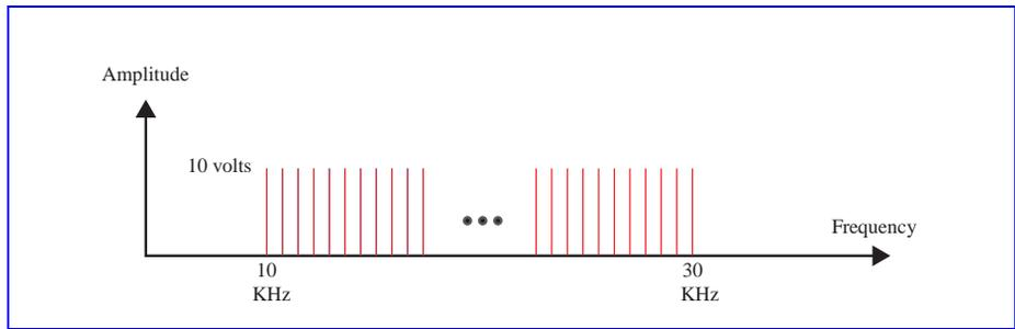
28. The signal is nonperiodic, so the frequency domain is made of a continuous spectrum of frequencies as shown in Figure 3.4.
