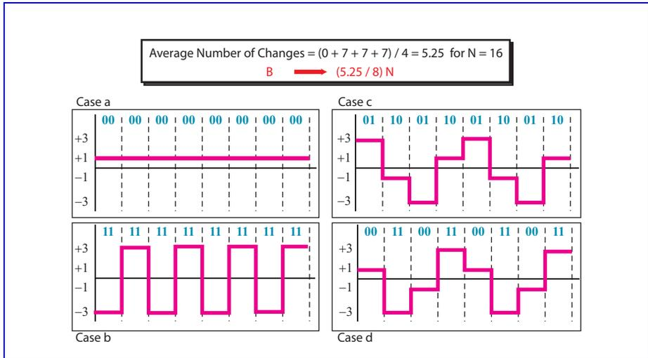
20. See Figure 4.6. B is proportional to  $(5.25/8) \times N$  which is inside the range in Table 4.1 ( $B = 0$  to  $N/2$ ) for MLT-3.
