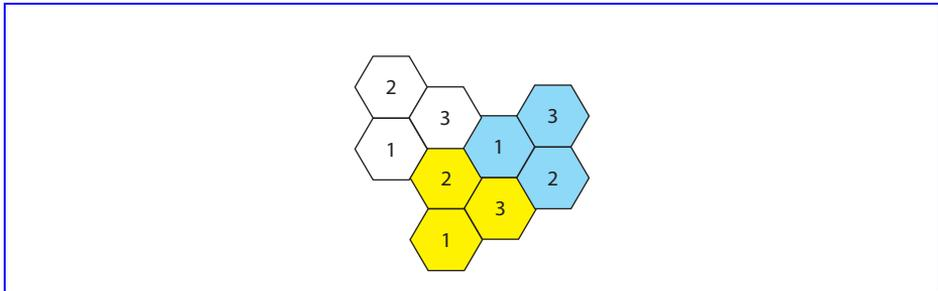
17. In *AMPS*, there are two separate bands for each direction in communication. In each band, we have 416 analog channels. Out of this number, 21 channels are reserved for control. With a reuse factor of 7, the maximum number of simultaneous calls in each cell is
