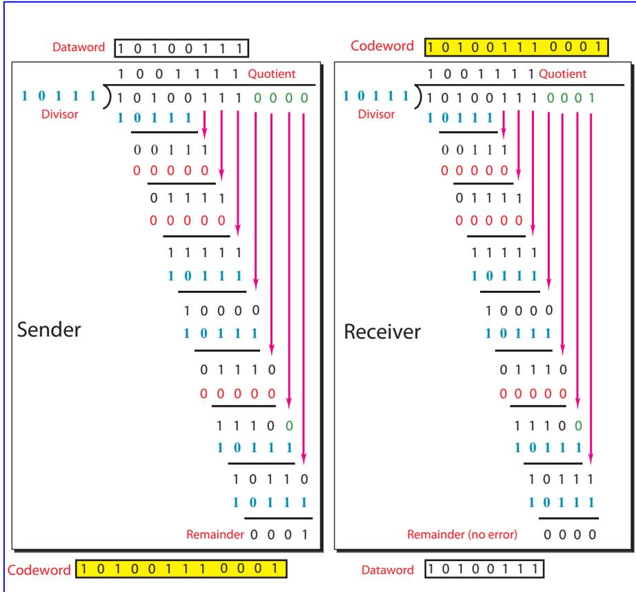
31. Figure 10.2 shows the generation of the codeword at the sender and the checking of the received codeword at the receiver using polynomial division.
