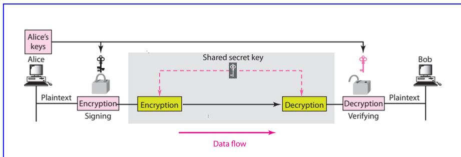
31. See Figure 31.6. The shaded area shows the encryption/decryption layer.
