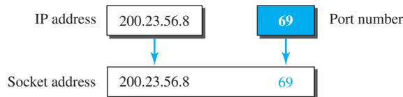
To use the services of the transport layer in the Internet, we need a pair of socket addresses: the client socket address and the server socket address. These four pieces of information are part of the network-layer packet header and the transport-layer packet header. The first header contains the IP addresses; the second header contains the port numbers.
